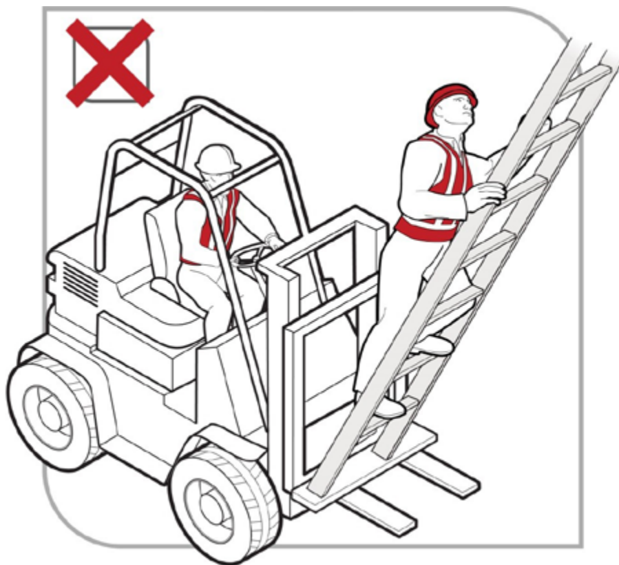
Figure 15 Unacceptable practice with ladder on forklift
