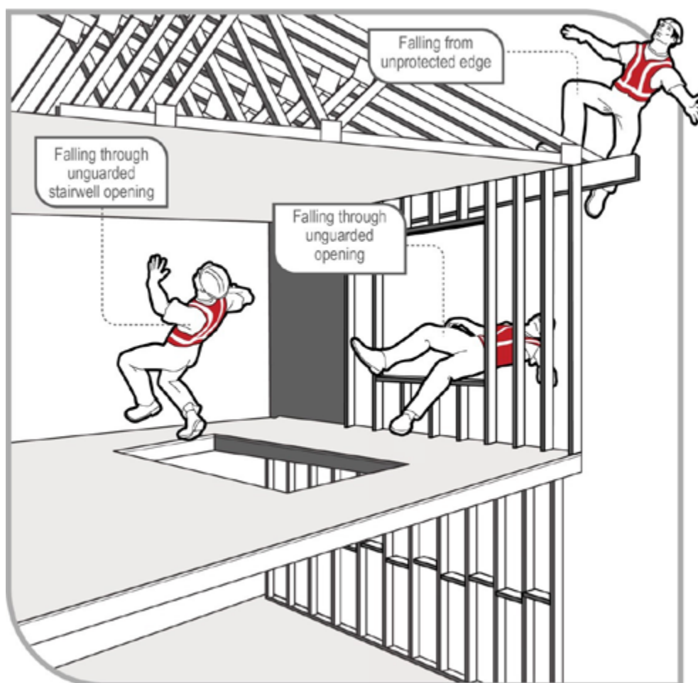
Figure 1 Examples of potential falls in the housing construction industry
